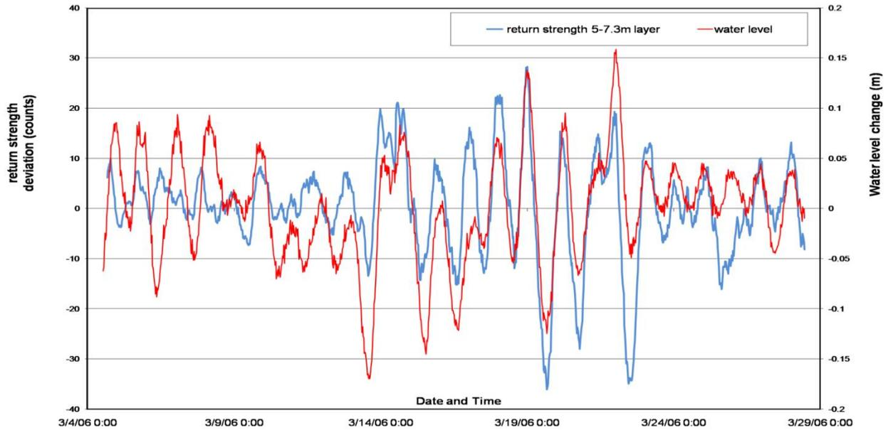
**Figure 4.** Deviations from mean March, 2006 SWIPS return strengths averaged over heights (relative to the riverbed) between 5m and 7.3 m and local water levels after filtering to remove variability on time scales  $> 24$  hours.
