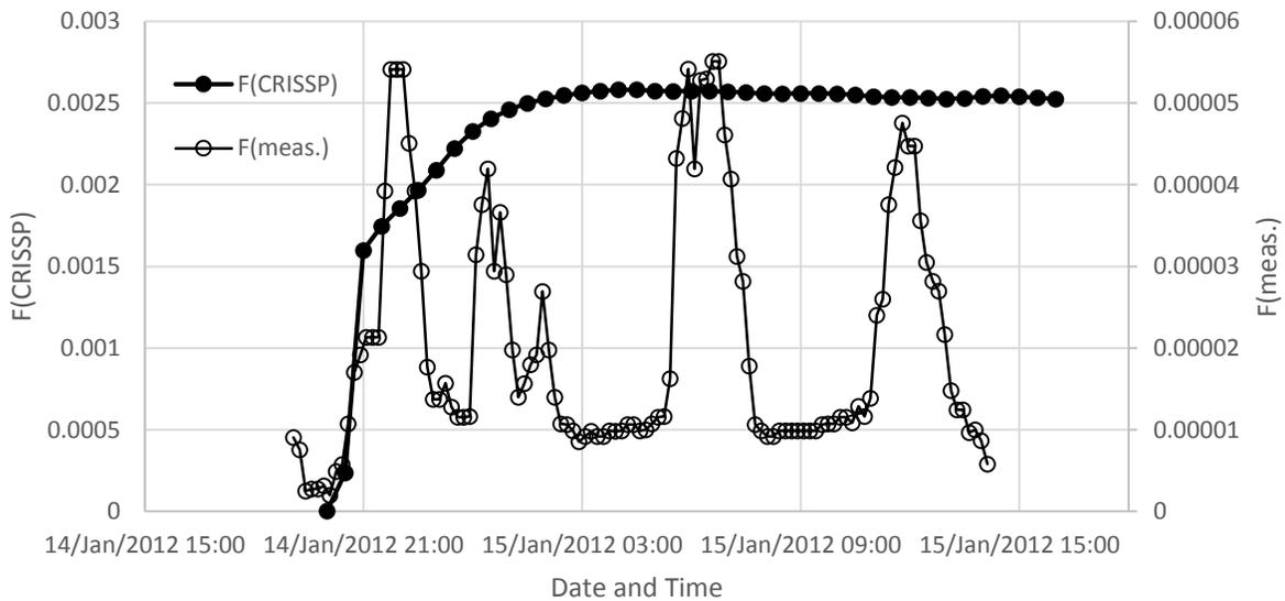
**Fig.5.** Comparisons of Interval 3 fractional volumes (Marko et al., 2015) as measured ( $F(\text{meas.})$ ) and simulated as described in the text ( $F(\text{CRISSP})$ ). The simulation results denote water column mean values while measured data represent mid-water estimates 2.3 m above the SWIPS instrument.
