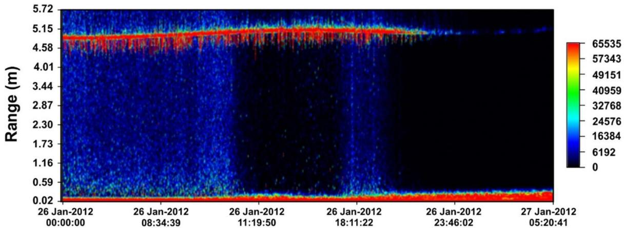
Fig. 7. Echogram of the 774 kHz SWIPS returns in the first blockage event of the 2011-2012 Peace River Study Program.
