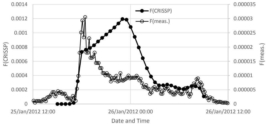
Fig. 6. Comparisons of Interval 4 fractional volumes (Marko et al., 2015) as measured (F(meas.)) and simulated as described in the text (F(CRISSP)). The simulation results denote water column mean values while measured data represent mid-water estimates 2.3 m above the SWIPS instrument.
