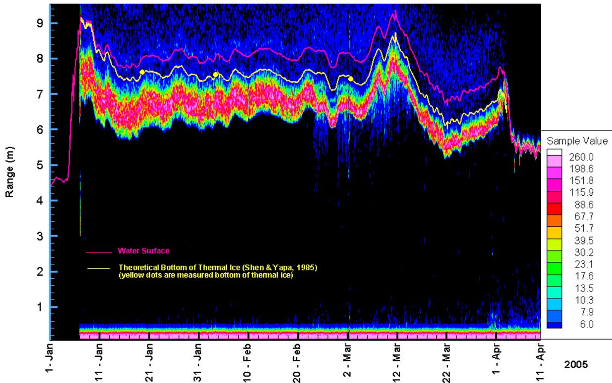
Fig. 3. Two-hour averaged SWIPS Profile return strength data acquired at 235 kHz over the mid-winter, January-April, 2005, stationary ice covered period. Also shown are local water levels and positions of the modelled, and measured (on 3 dates) lower surface of the thermal ice.
