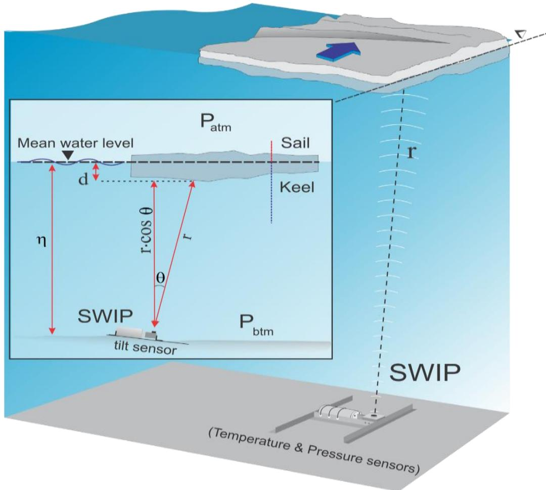
Fig. 1 Simplified sketch of deployed (single frequency) SWIPS unit and standard range measurement parameters
