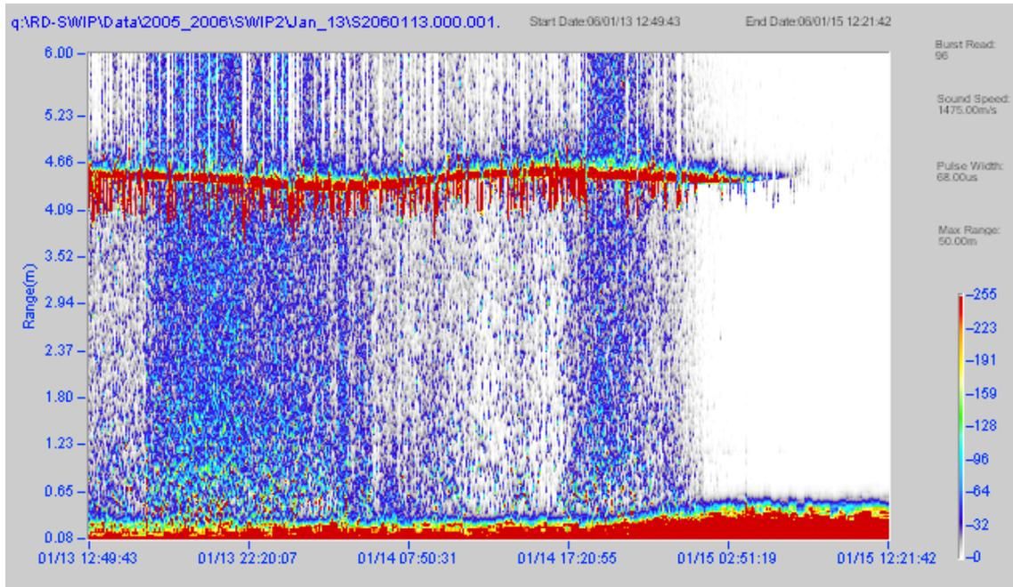
Fig. 2. SWIPS Profile return strength data acquired at 546 kHz prior to and during a Jan. 2006 frazil interval.
