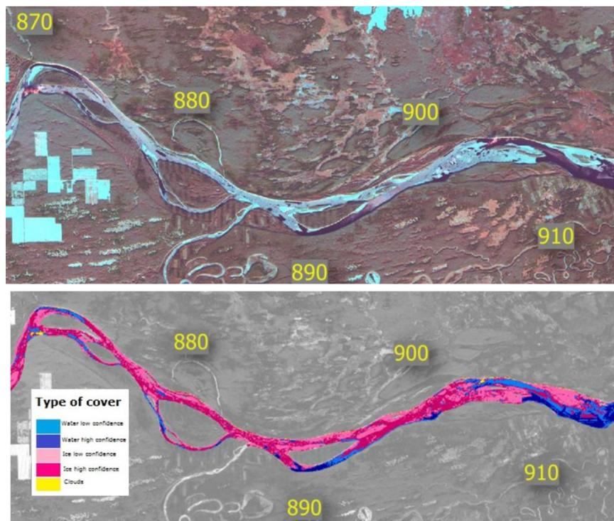
Figure 3: Top: RGB composite of a section of the Landsat-8 image of November 11th, 2014. Bottom: Classification resulting from IceFRONT.
