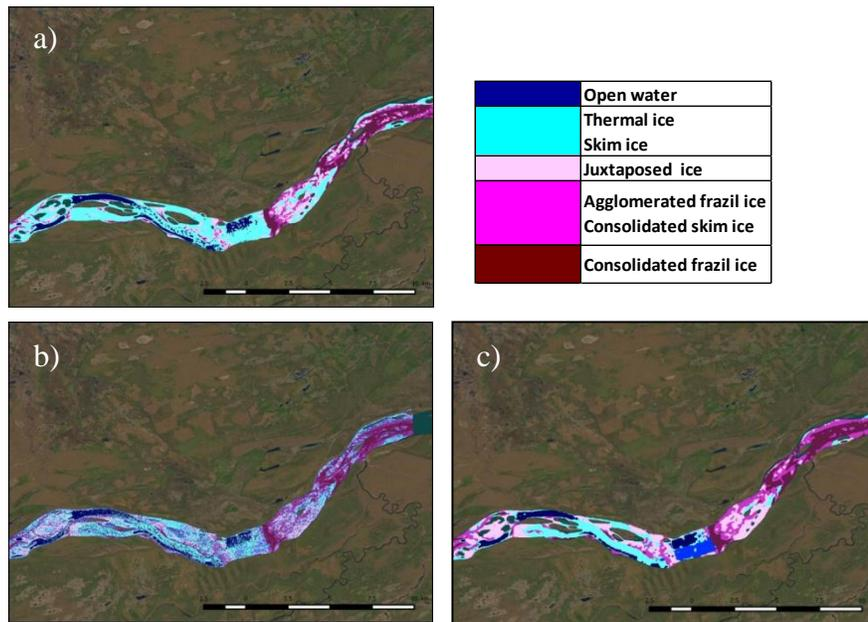
Figure 5: Classification of ice types from three methods a) IceMAP-R; b) Alpha/Entropy; c) Kennaugh elements.
