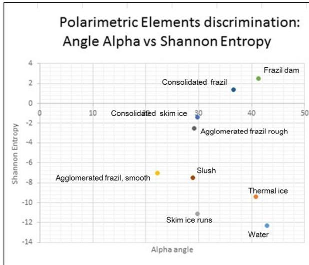
Figure 4: Defining thresholds for classification of ice types from polarimetric parameters.
